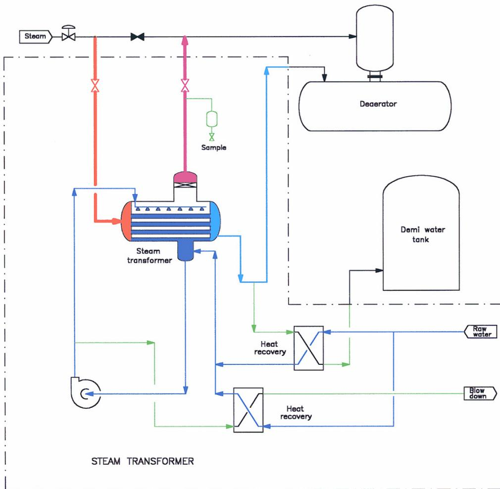
Fig. 1. Process flow scheme of the Busto Arsizio project.
